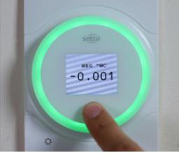
If the DISPLAY is set to "OFF", the LCD display will display Setra logo under normal operation. To see a digital pressure reading, simply press on the lens of Setra Filter Alert.
