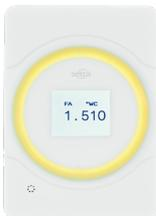
If pressure exceeds the warning limit threshold, the LED light ring will glow yellow, indicating that the filter should be changed soon. If pressure exceeds the alarm limit threshold, the LED light ring will glow red, indicating that the filter should be changed as soon as possible.
