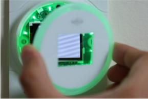
In the event Setra Filter Alert needs to be removed for service, first remove the front lens. To remove the front lens, grab the front lens from the left and right side edges, and pull the lens away from the wall.
