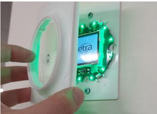
7. Install the faceplate by firmly pressing it into place over the base unit housing. **Note: Press the plate in at a slight angle, leading with the bottom edge.**
