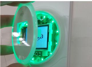
8. After configuration is completed align and engage the top two snaps. Then, align and install the front lens to the faceplate by inserting top snap first, followed by the bottom snap. Left and right snaps are alignment only.
