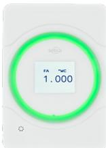
Under normal operation with pressure within the configured alarm limits, the LED light ring will glow green. Or, NOT be illuminated depending on light ring configuration chosen during setup.
