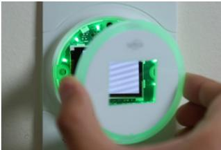
With the unit powered on, grab the lens by the left and right edge, then pull away from the unit.
