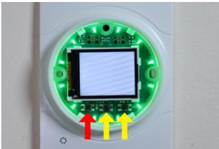
Locate the 3 buttons located below the LCD display.
