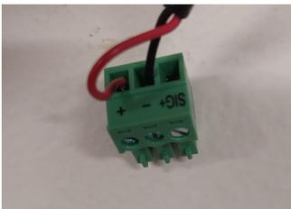
2. Add connector to the in-wall wiring for power and analog output (if required) per section 7.0. Attach the power connector to the Filter Alert and the intermediate tubing to the in-wall tubing.
