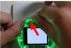
Next, locate the 4 snaps holding the faceplate to the unit. Carefully push on the inside lip of the faceplate near each snap to disengage each snap one at a time.
