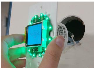
3. As you push the Filter Alert unit into the electrical box or wall, push the tubing into the conduit tube or wall cavity.
