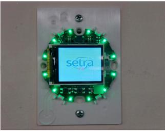
4. Push Setra Filter Alert into the wall or enclosure and secure with two (2) mounting screws.
