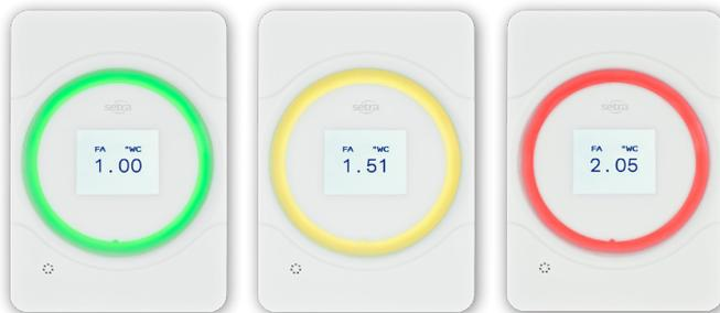
Setra Filter Alert features an LED light ring that changes color based on the pressure differential and the user defined thresholds. The light ring will glow green when the filter health is good, yellow when the filter needs changing soon but is still acceptable for use, and red if the filter needs to be replaced.
