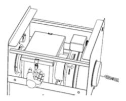
8. Remove the HEPA filter for ease of access to the UV bulbs. Remove UV bulbs from their boxes, handling only by the white packaging to protect bulb life.
